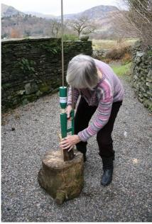
First take hold of the handle, slide it (and the weight above it) up the pole and position the log under the blade, so the blade rests on it and holds it in position.
