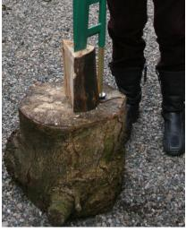
Next slide the weight to the top of the pole and let it drop down onto the blade. This will drive the blade into the log, and may split the log on the first attempt. If it doesn't work first time just slide the weight back up the pole and drop it again. For large logs, or those with knots in, it will take a few goes before the log splits.
